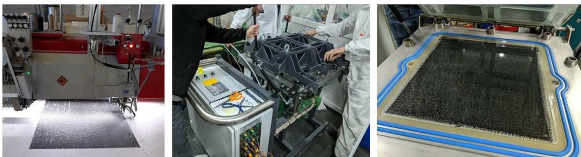
Fig. 1: PWF1 embroidering process, RTM equipment and composite plate obtained
